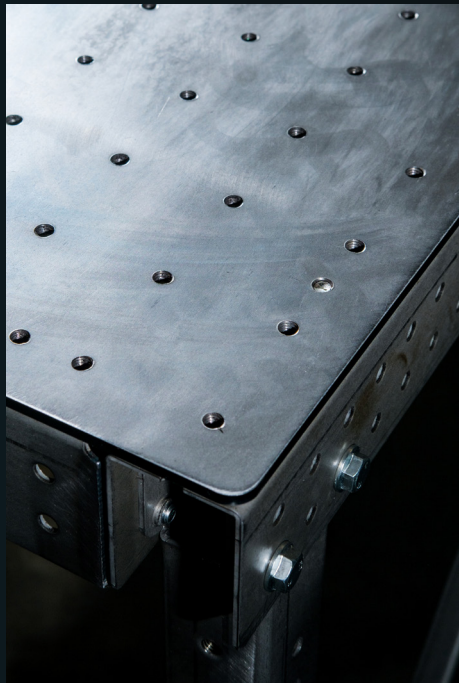
Detail of the welding table top with tapped M8 holes.
