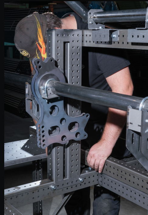
View of our rear end jig with 4-link plate for the doorslammer kits.
